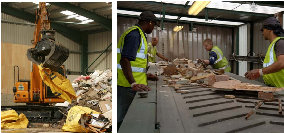
Figure 2.6 Emptying of HIPPOBAG™ using grab and manual sorting of materials at a Waste Transfer Station.
